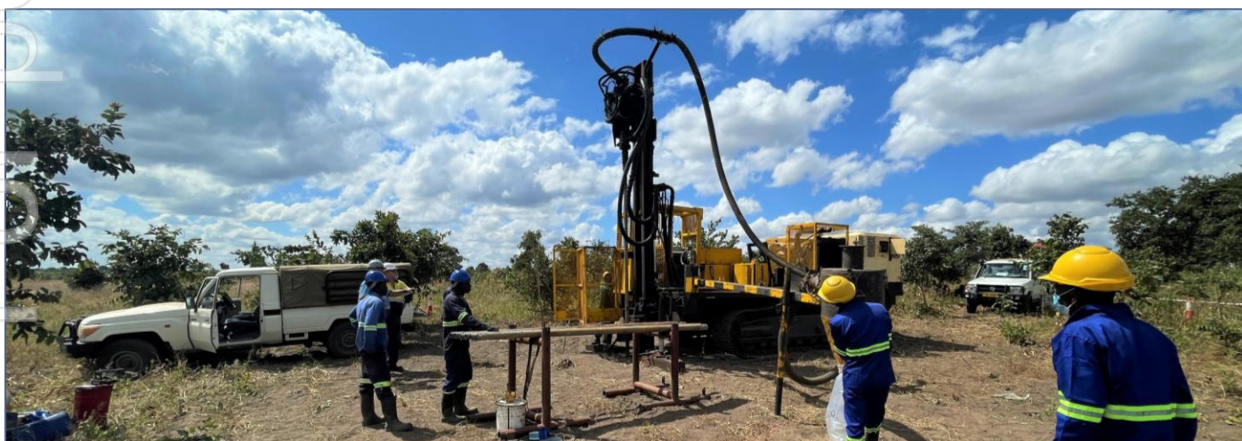
Figure 5: Air-core (AC) drilling at Kasiya in May 2022.
