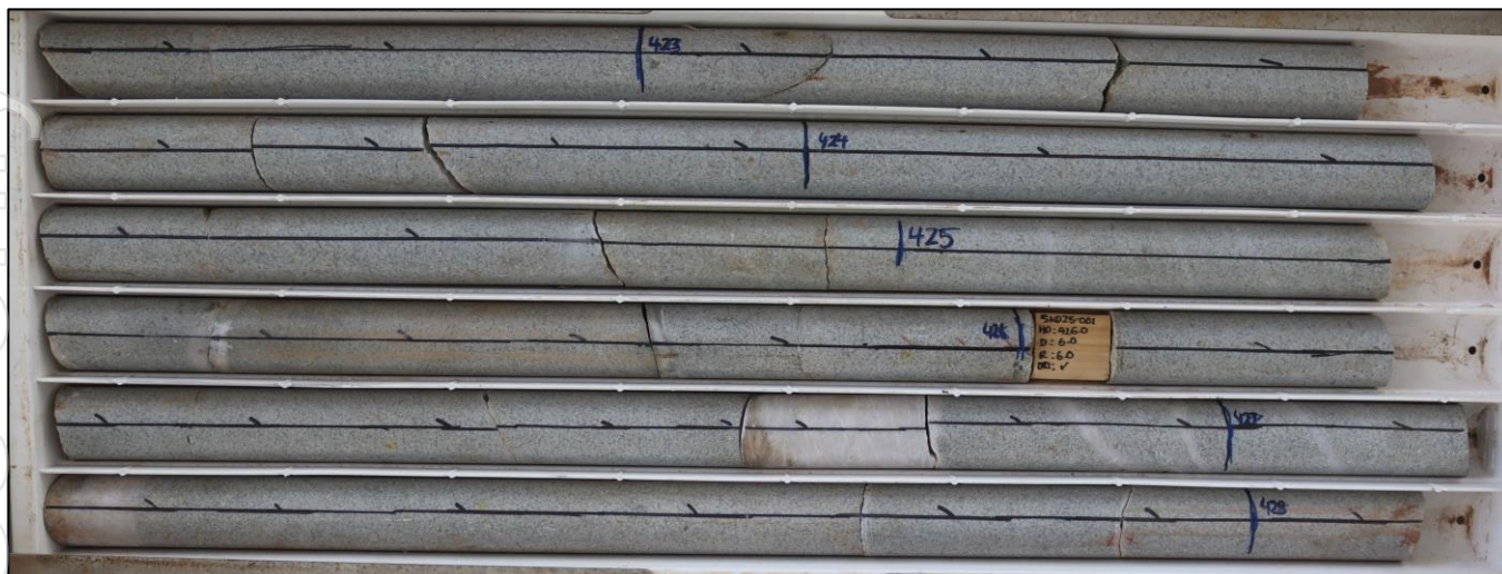
Figure 6: Core photo from drillhole SND25-001, including an intercept of 2m @ 41.3g/t Au from 425m. Mineralisation is hosted by sheeted discrete quartz veins displaying weakly sericite-altered haloes, within a Tonalite intrusion.
