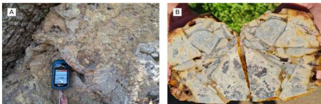
Figure 5 – Examples of hydrothermal breccia samples collected in the Mount Quandong area. (A) DTRC204 - Outcrop of brecciated, strongly clay-silica altered volcanic with spongy boxworks after ex-sulphides; (B) DTRC188 - Sample of brecciated, silica-clay altered volcanic with quartz-hematite and minor pyrite infill.
