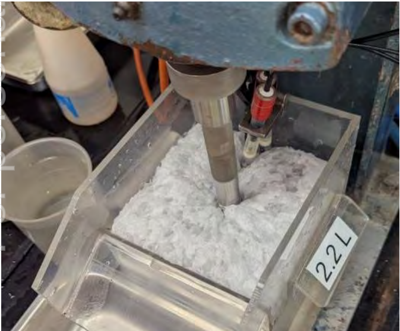
Figure 46: Typical fresh ore cleaner flotation trial.
