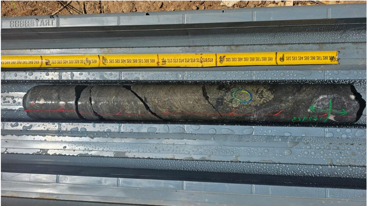
Figure 2: Diamond drill core (HQ) from hole CMKN1004 from 230.4m to 230.9m, showing a ~50cm massive sulphide vein comprising approximately 85% pyrite, arsenopyrite and proustite, hosted within sheared rhyolite porphyry.
