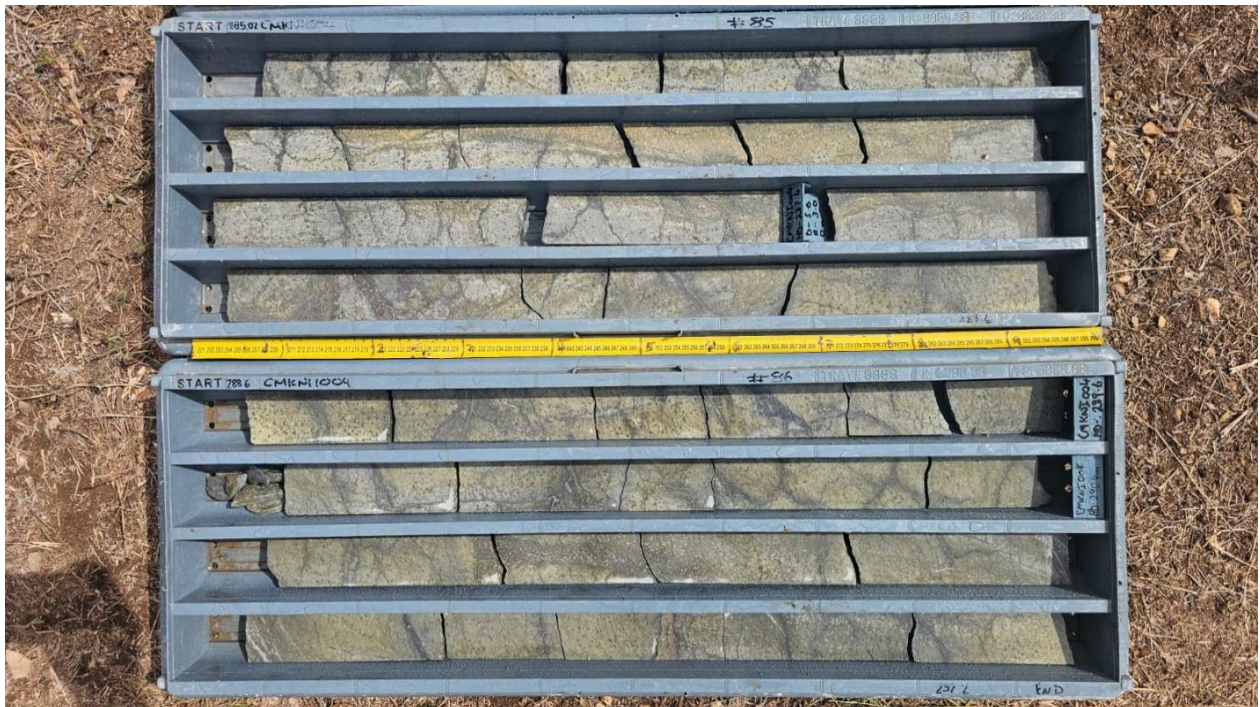
Figure 3: Diamond drill core (HQ) from hole CMKN1004 from 285.02m to 292.2m, showing stockwork style arsenopyrite-pyrite-proustite stringer veins within sericite-altered rhyolite porphyry.
