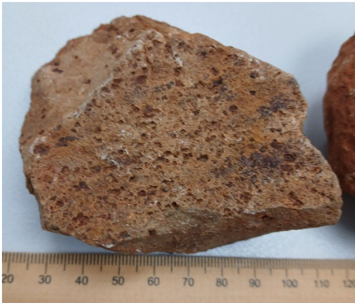
Figure 3 Close up image of an unremarkable looking Albitite grading up to 12.04g/t Au on surface
