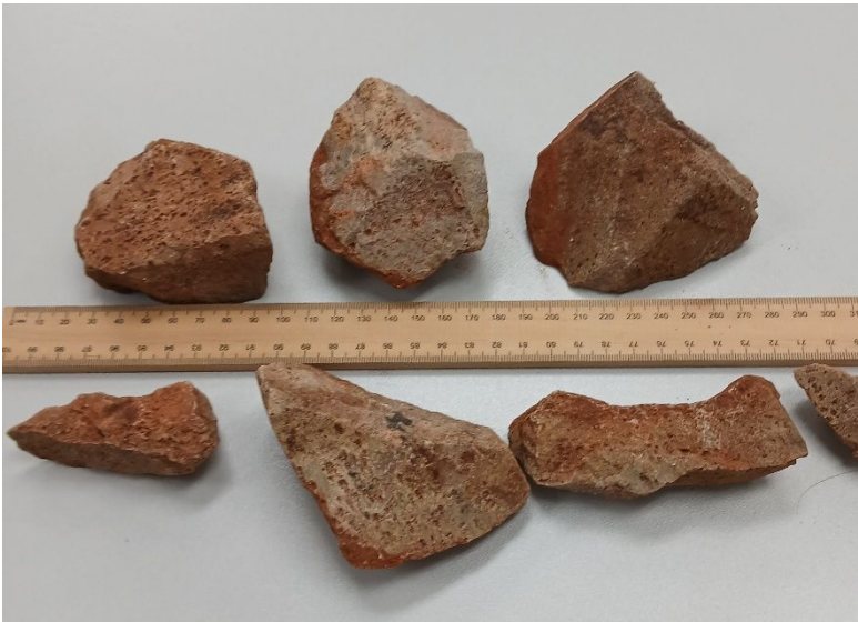
Figure 2 Image displaying abundant rock fragments of albitite with sulphide casts
