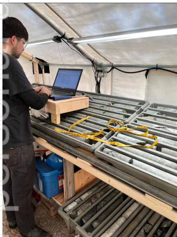
Figure 2 – Core logging and sampling preparation
