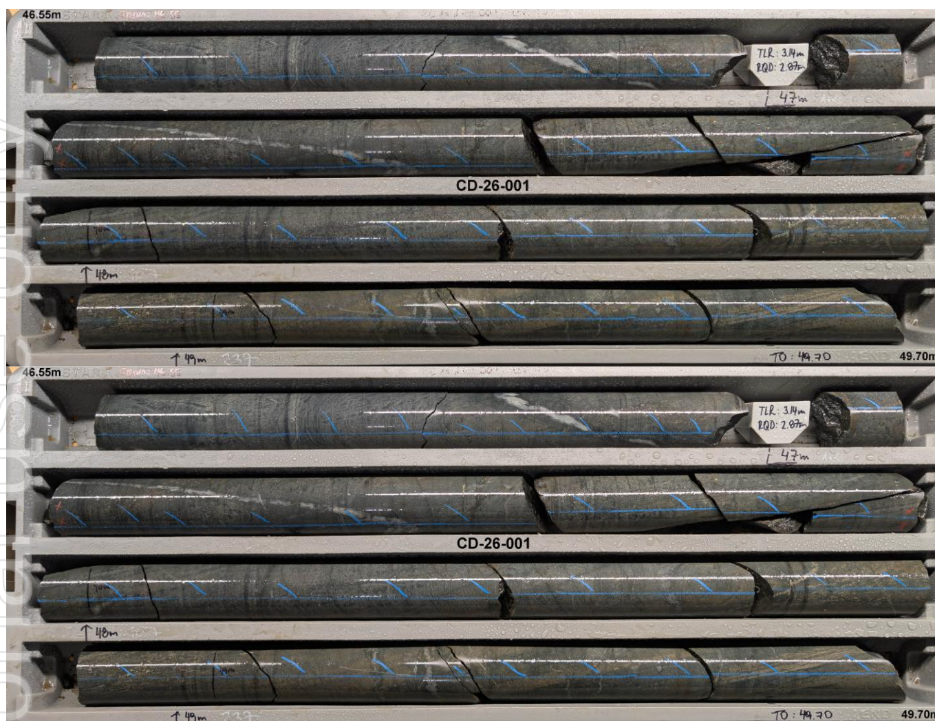
Figure 1 Diamond Drill Core from CL-26-001 (BIF with sulphide mineralisation)
