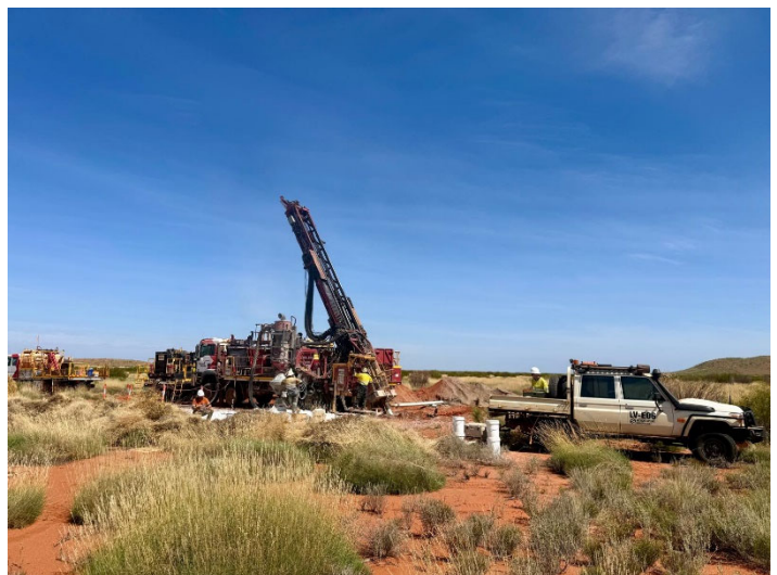
Photo 1: RC drilling at the Elsa Gold-Copper Prospect – Paterson Province WA
