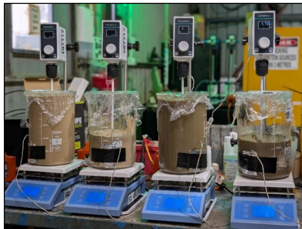
Figure 2: Stirred vessel leach apparatus
