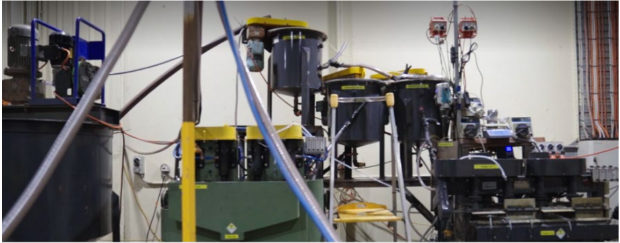
Figure 10-3: Continuous REE flotation pilot plant at Nagrom in Western Australia
