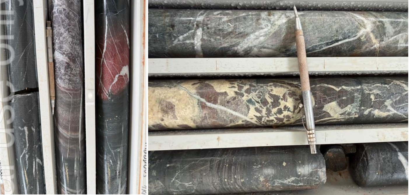
Photo 4 & 5: Magnetite – hematite & pyrite alteration in bedded siltstone and breccia zone (MBDD003; 495 - 498m).
