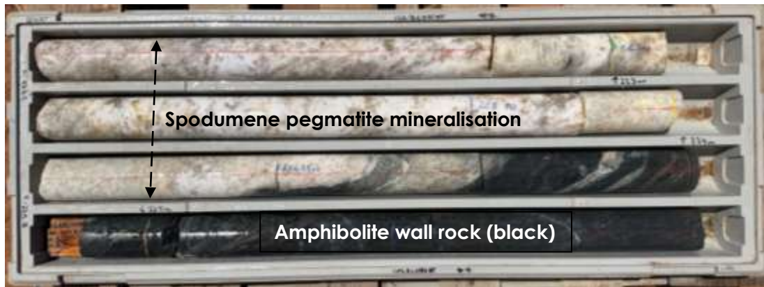
Photos 1 and 2. Coarse-grained spodumene in diamond drill core from CLMRC055DT from 220m to 224.35 with an average grade of 1.33% Li 2 O and 74ppm Ta compared to the amphibolite wall rock.
