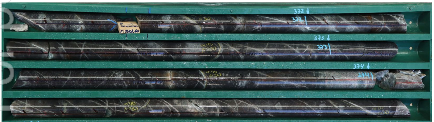
Photo 2. Zone of intense pyrite and quartz vein stockwork with fine disseminated pyrite 372m downhole in 26LHDD073* (refer to Appendix 1).
