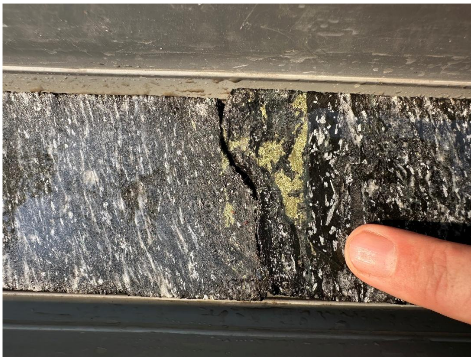
Figure 3. Copper mineralisation from drill hole MWDD001 (33.9-34.0m) in biotite-rich kyanite-schist
