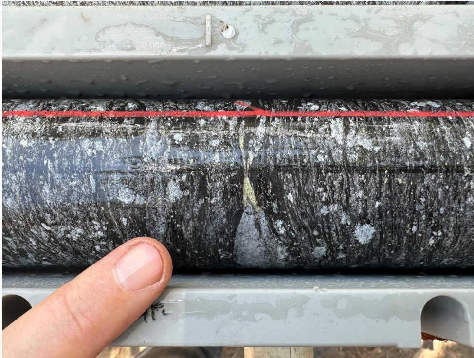
Figure 4. Copper mineralisation from drill hole MWDD007 (103.8-103.9m) within laminated schist-felsic gneiss
