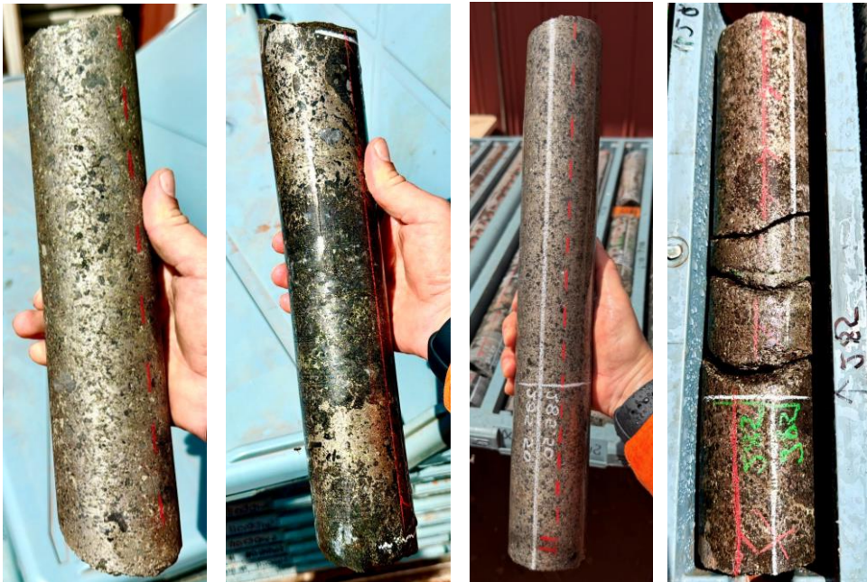
Figure 1. Massive to semi-massive sulfide intervals from SWDD011 at depths (from left to right) from 287.6m-287.85m, 288.15-288.45m, 285.2-285.65m, 284.9-285.2m.
