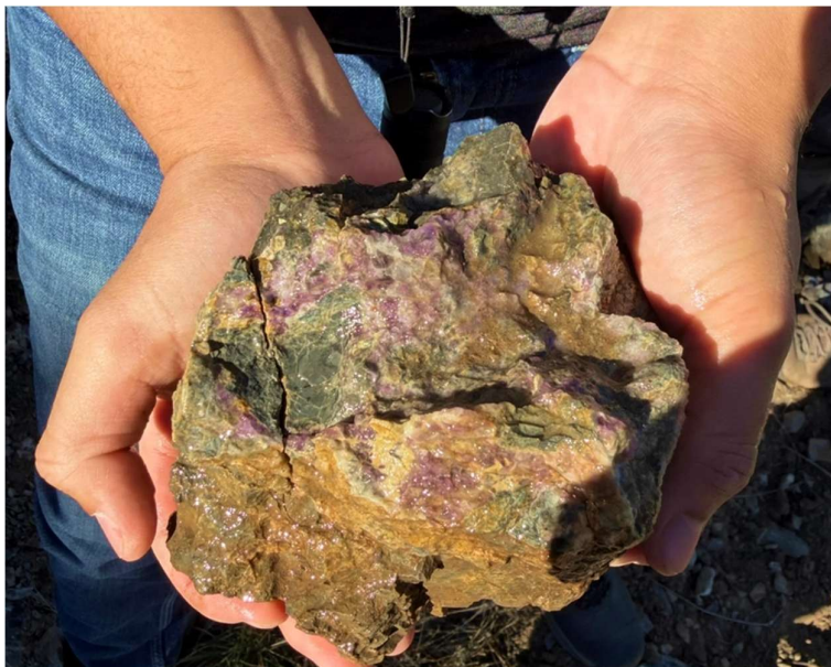
Figure 1 Sample QC260251 with purple and white fluorspar from the contact zone on west side of Mammoth
