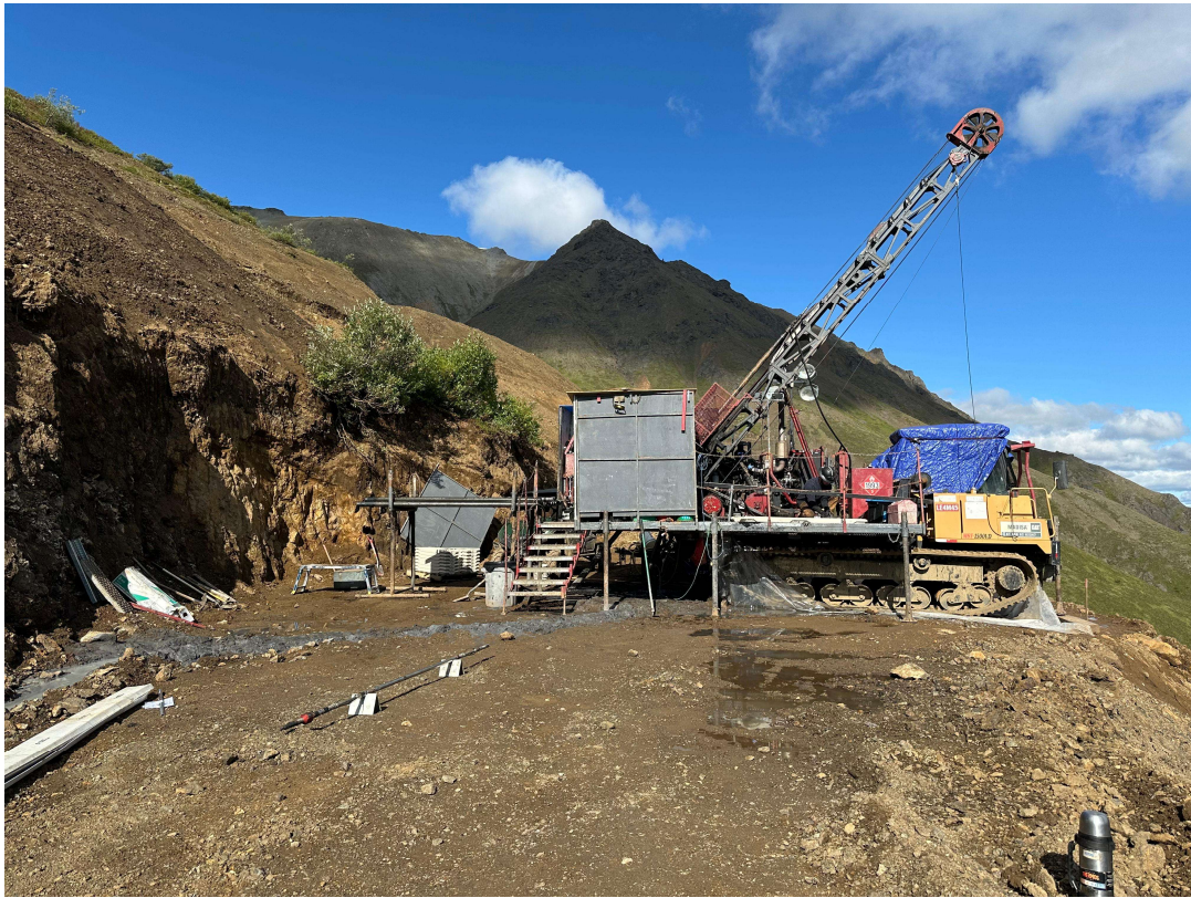
Figure 5. Diamond drill rig producing oriented diamond core at Caribou Dome (CD25-001).
