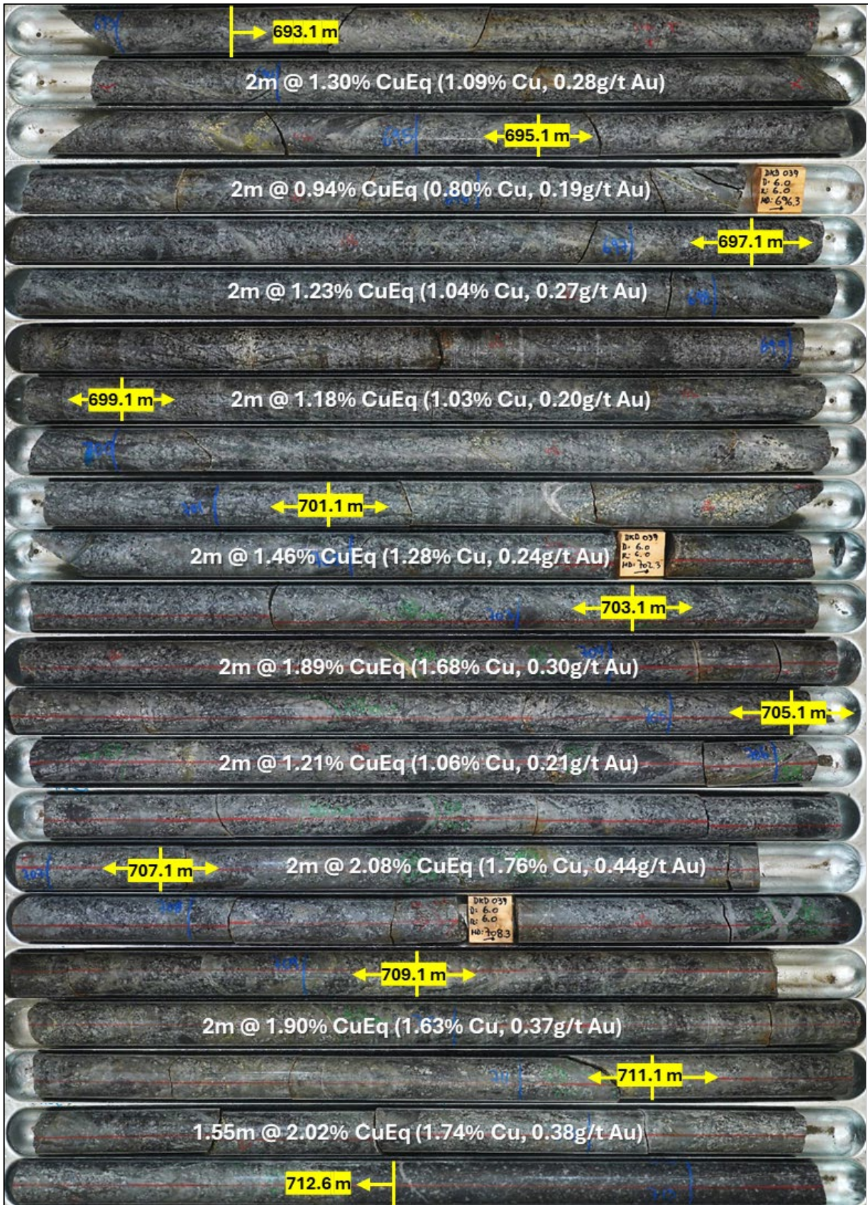
Figure 5. Core photos for DKD039 showing high-grade zone of 19.6 m grading 1.51% CuEq (1.30% Cu, 0.29g/t Au, 2.26g/t Ag) from 693.1 m within the broader high-grade zone 61.5m grading 1.03% CuEq (0.90% Cu, 0.18g/t Au) from 670.7 m.
