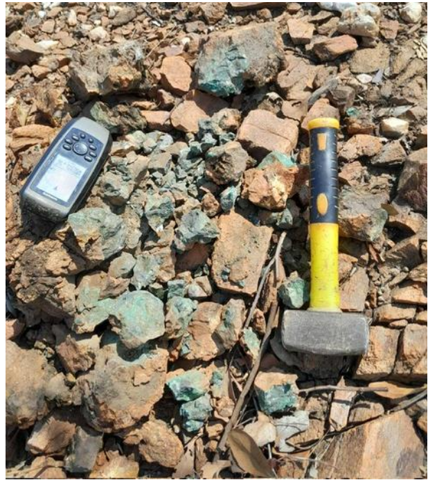
Photo 1 & 2: Copper carbonate outcrop along the northwest - southeast fault surveyed by IP (Red Devil). Sample ID – BDR033: 40.1% Cu, 27.8g/t Ag & 0.113g/t Au.
