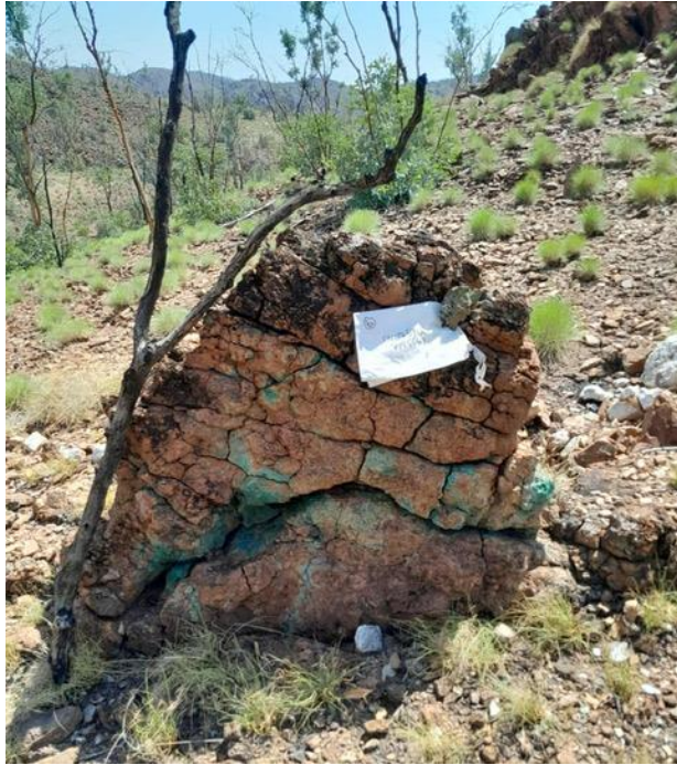
Photo 1 & 2: Copper carbonate outcrop along the northwest - southeast fault surveyed by IP (Red Devil). Sample ID – BDR033: 40.1% Cu, 27.8g/t Ag & 0.113g/t Au.
