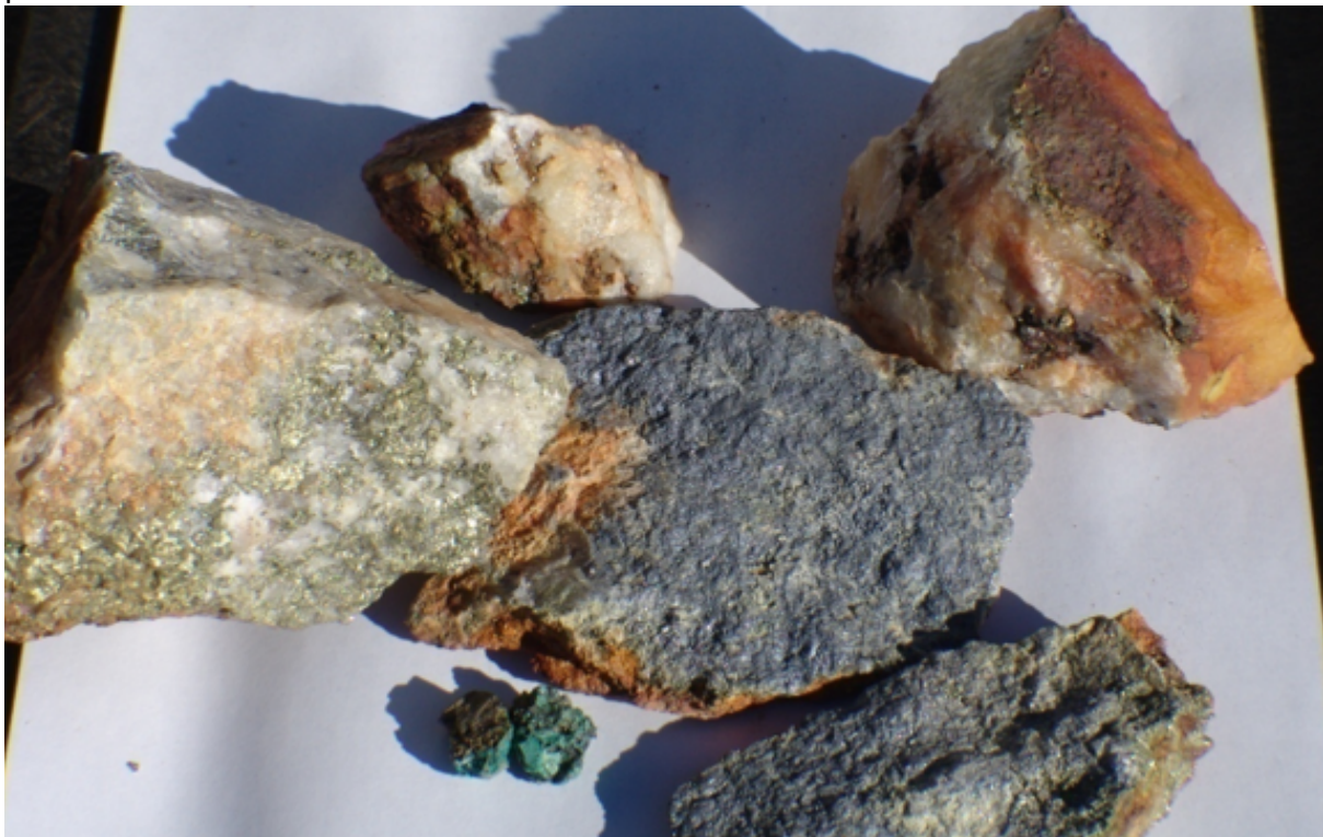
Figure 4: Sample 25LRX001 showing Molybdenite ( \text{MoS}_2 ), Chalcopyrite ( \text{CuFeS}_2 ), Azurite ( \text{Cu}_3(\text{CO}_3)_2(\text{OH})_2 ), some Malachite ( \text{Cu}_2\text{CO}_3(\text{OH})_2 ) and abundant Muscovite ( \text{KAl}_2(\text{AlSi}_3\text{O}_{10})(\text{OH})_2 ).
