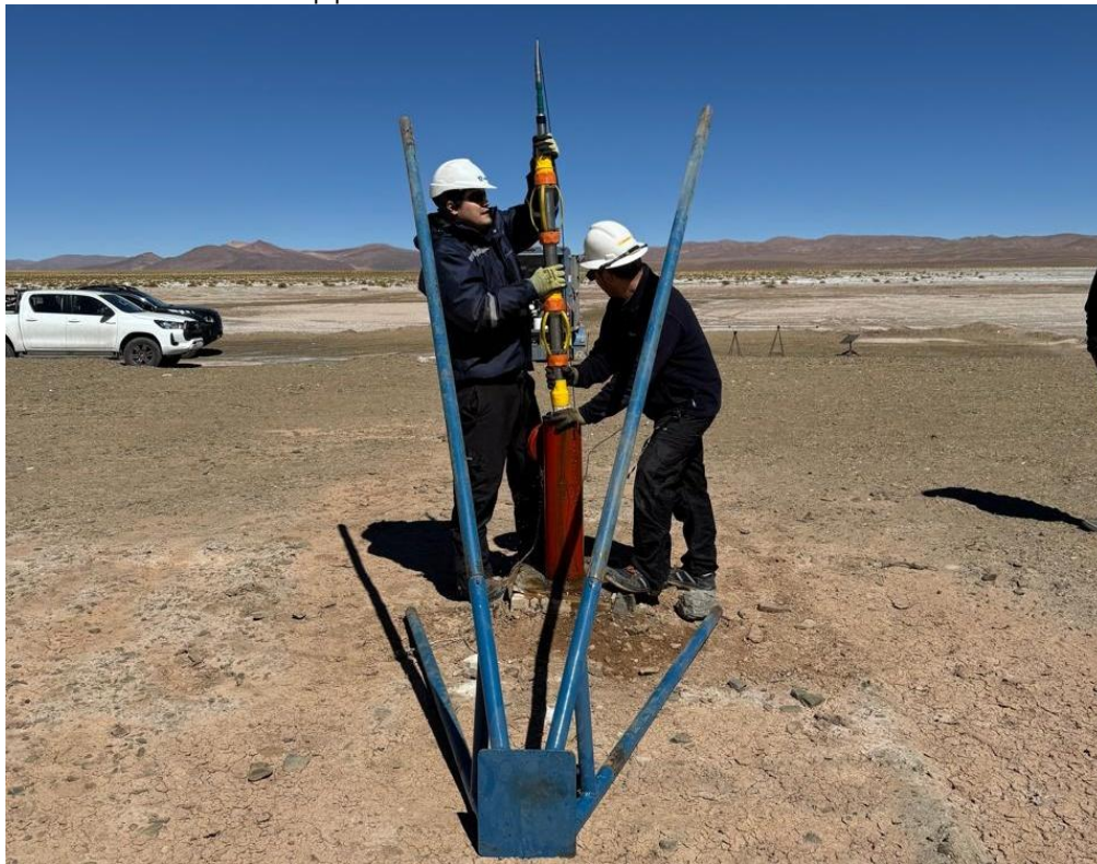
Figure 1. Permanent magnet and antenna that are lowered into a borehole to record the response of the nuclear magnetisation associated with hydrogen nuclei in the pore fluids (e.g., groundwater) of the formation.
