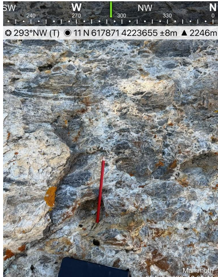
Figure 4 Close-up view of main fluorspar replacement body in the area of channel QCCH2602_4. The white material is fluorspar, and the grey material is fluorspar impregnated in limestone (pencil for scale)
