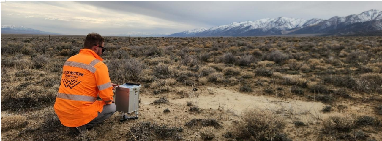
Figure 1; Photo showing field data collection using a Scintrex CG 5 gravimeter at the Linka Project, Nevada, USA.
