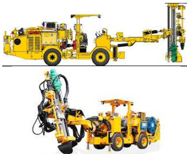
Figure 1 Muki Production Drilling Rig
