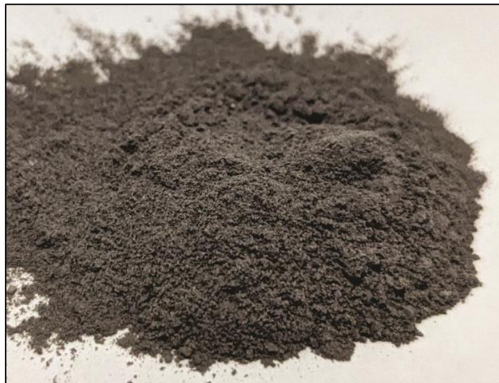
Figure 3: Antimony sulphide (37% Sb) precipitated from leach liquor 6
