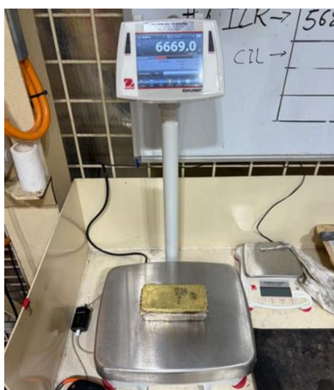
Figure 2: Total 214oz (6,669g) doré bars BJM049 and BJM050 – smelt at Blackjack on 8 th April 2026. Internal assay returned BJM049 at 78% purity.
