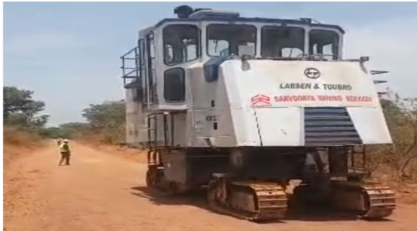
Image 3 and 4: Surface Miner Arriving on Site
