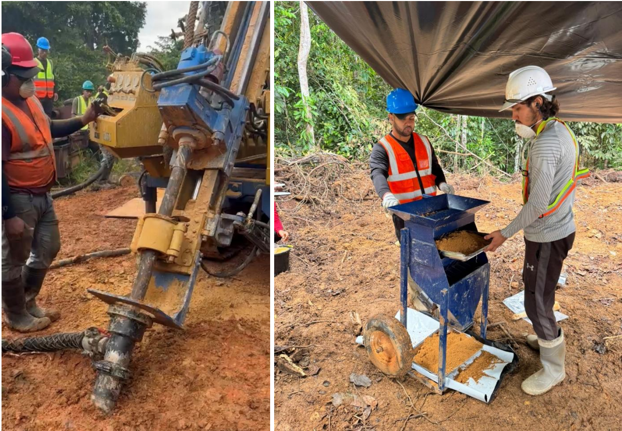
Figure 3: Current RAB drilling ongoing at North Peters (Left), riffle splitter for RAB drilling (right)
