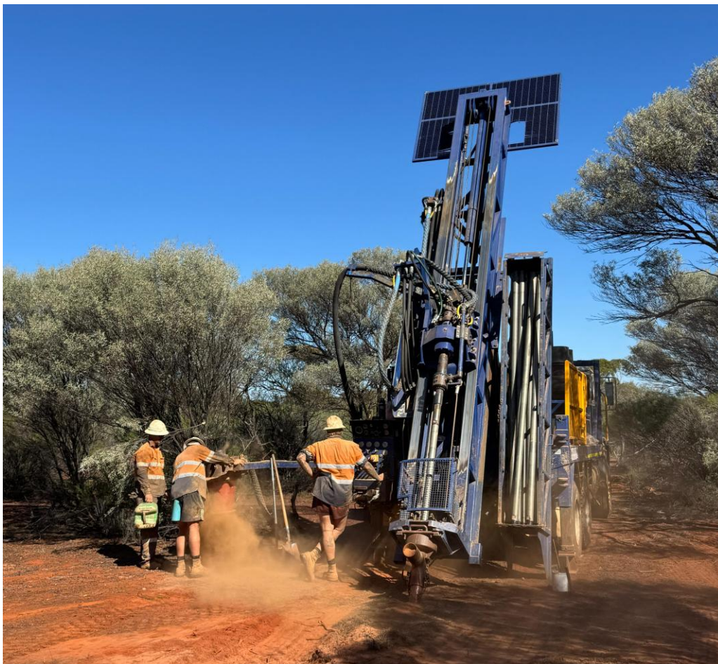
Figure 1: Aircore drilling at the Fluffy Prospect
