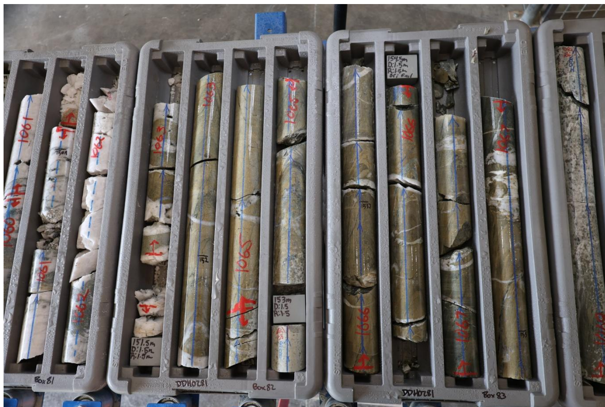
Figure 3: Consecutive Core trays 80-83 of prospective gold mineralisation in DDH0281 marked for cutting and analysis; Main zone of interest was noted from 144.5-155.4m, within a wider 20m zone of alteration and veining from 144.5-164m downhole.
