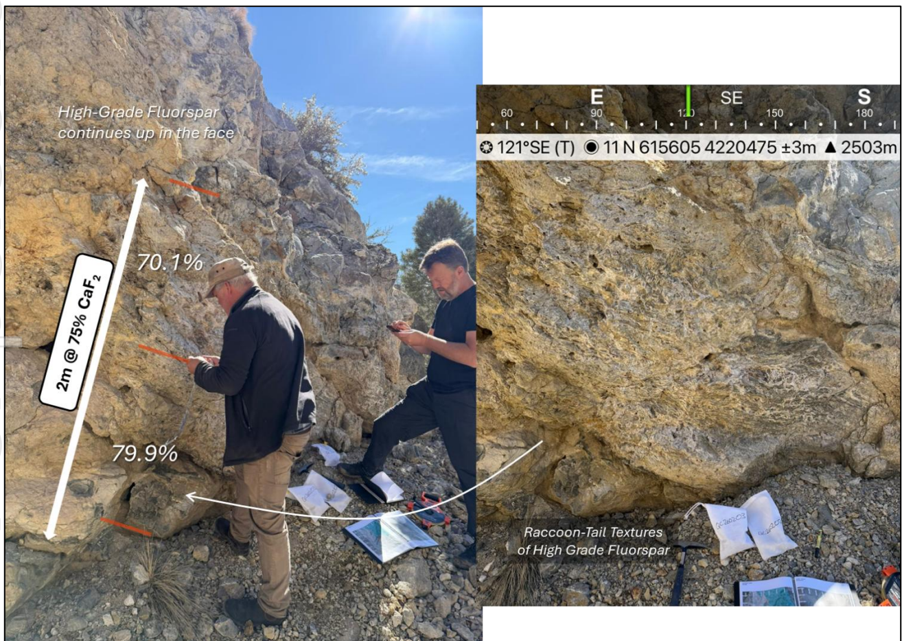
Figure 5: View SE of in-pit (channel QCCH2602_1) sampling at Horseshoe. Orange marks indicate 1m samples. Only the reachable extent of the outcrop was sampled. This outcrop displayed "Raccoon Tail" textures of banded fluorspar – a classic epithermal replacement style in high-grade fluorspar deposits.
