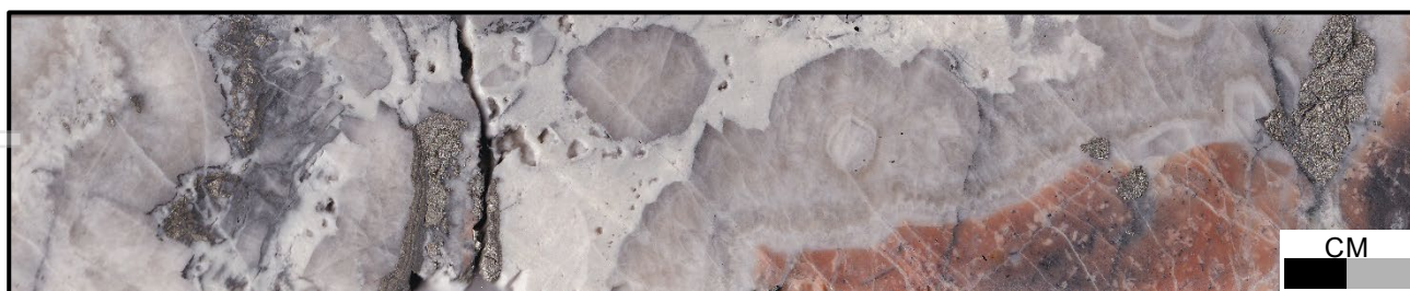
Figure 3: SPD025 667.8m grading 0.96 g/t Au . Low sulfidation epithermal crustiform veining with oatmeal texture and layered pyrite bands, and late pyrite overprint.
