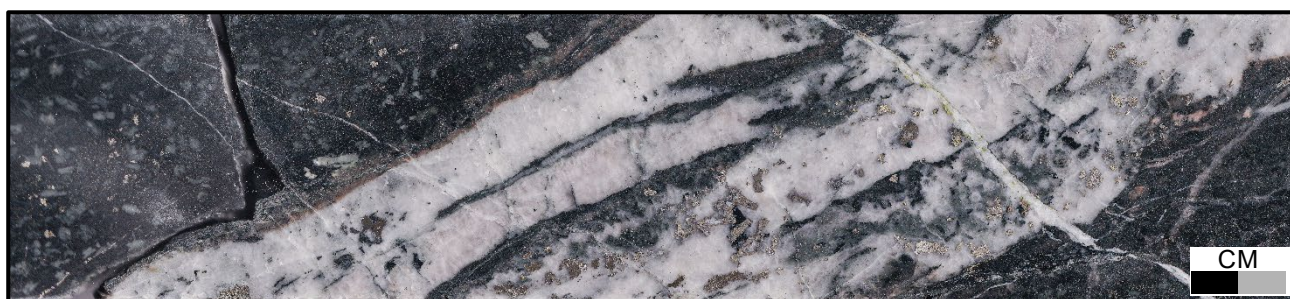
Figure 6: SPD029 58m grading 3.75 g/t Au . Laminated carbonate-pyrite-chalcopyrite-chlorite vein overprinted by carbonate-epidote vein in monzonite with disseminated pyrite halo.
