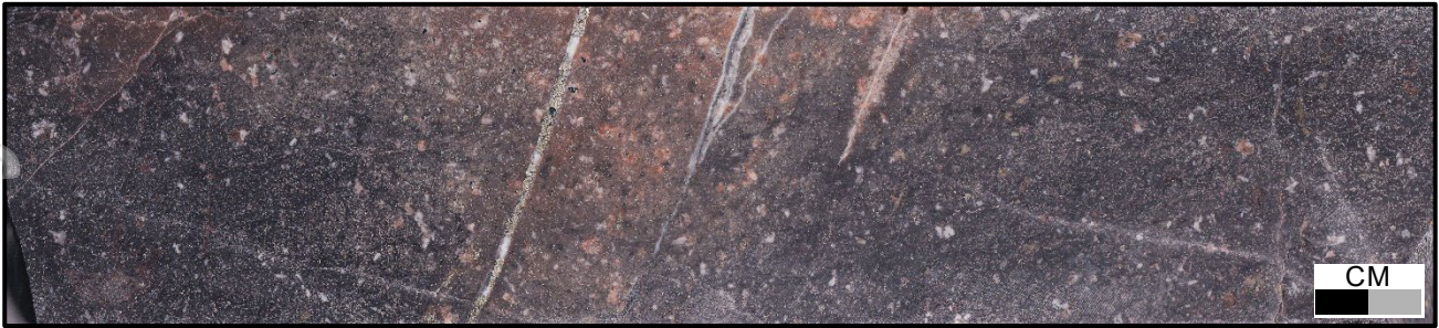
Figure 4: SPD024 512.2m grading 1.59 g/t Au. Pyrite-carbonate and quartz-pyrite veins in weakly potassic altered andesite.
