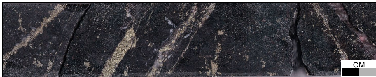
Figure 2: SPD025 491m grading 47.81 g/t Au . Pyrite, Chalcocopyrite and pyrite-chalcocopyrite veinlets, quartz-pyrite-chalcocopyrite veins and disseminated pyrite in basalt.
