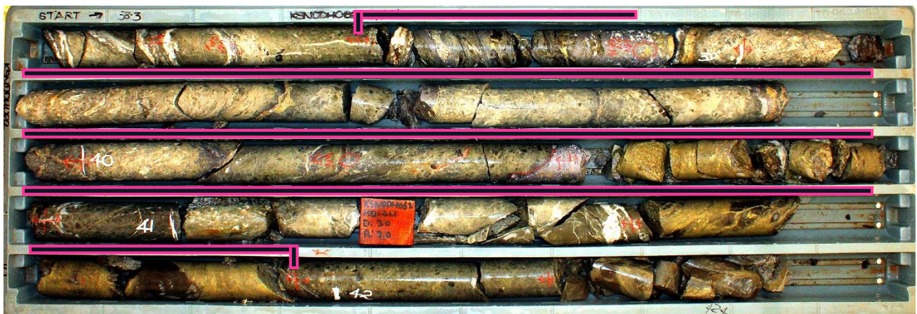
Figure 1: Massive sulphide component of the 7.5m interval from 38.6m in hole KSNDDH062. Interval highlighted in pink; 3.4m @ 1.09g/t Au, 2.82% Cu, 6.86% Pb, 1.86% Zn, 77g/t Ag from 38.6m .
