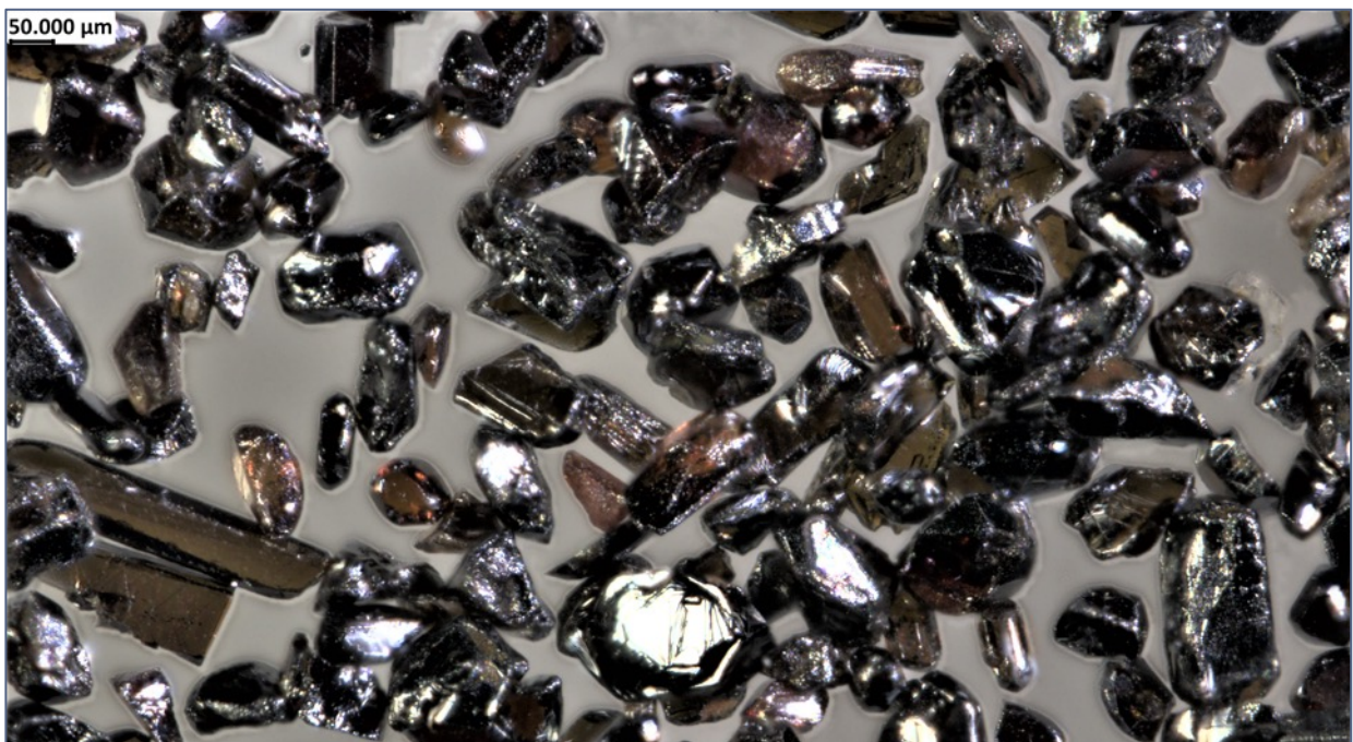
Figure 20: Photomicrograph of high-purity rutile product
