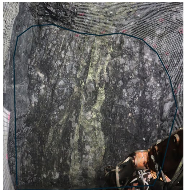
Photo 5: Left – cross section of Jericho Mineral Resource model at development face. Right – development face looking north along J1 lens development drive, showing visible copper sulphide mineralisation. Face dimensions are approximately 5.5m wide by 5.5m high*.
