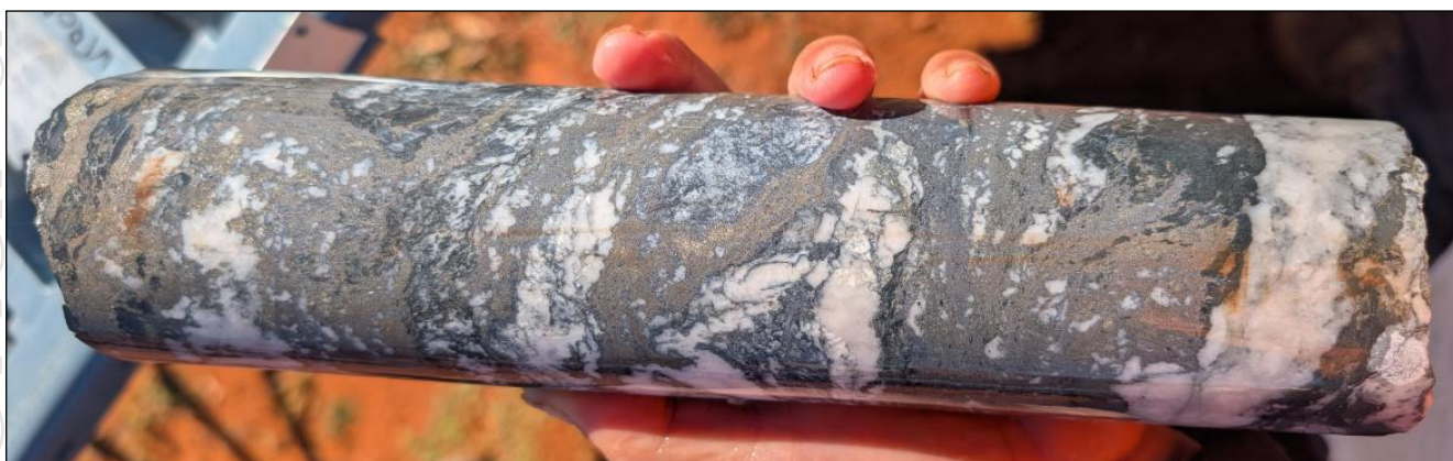
Figure 1 – Semi-massive/stringer sphalerite-galena-pyrite mineralisation @ 546.3m down-hole
