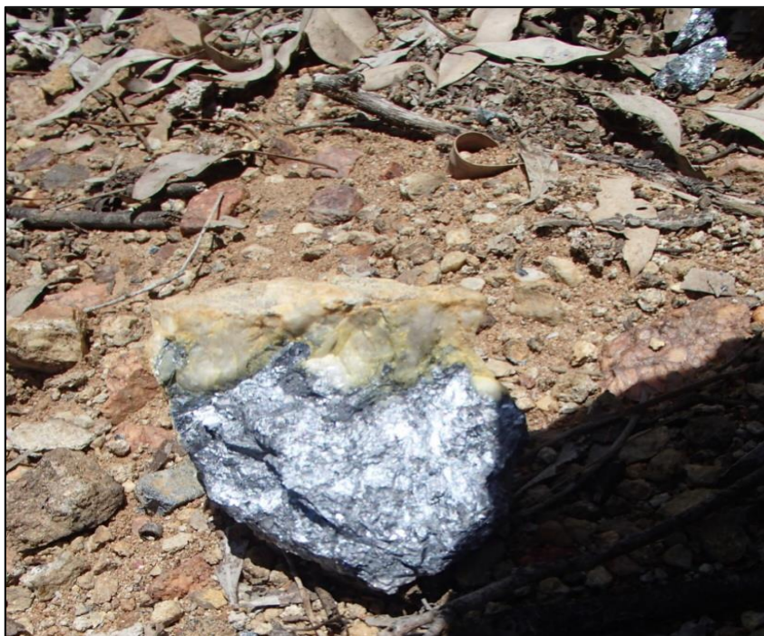
Figure 7: Banshee mine waste dump material observed (unsampled) by Dart Mining in January 2025 showing antimony mineral (70% stibnite*) with encasing vein quartz.*
