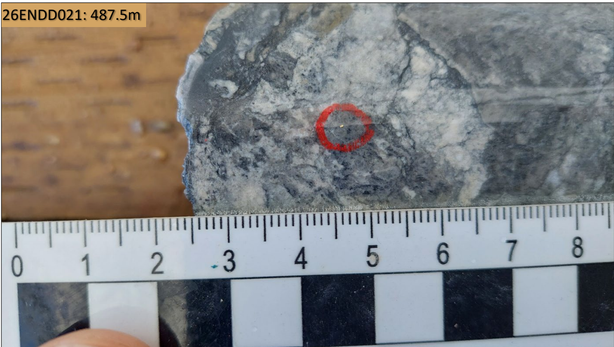
Photo 3. Visible gold (circled red) in hole 26ENDD021 at 487.5m down hole in brecciated quartz-carbonate-pyrite-arsenopyrite veins within brecciated/faulted granite. Numerical units on scalebar are centimetres.
