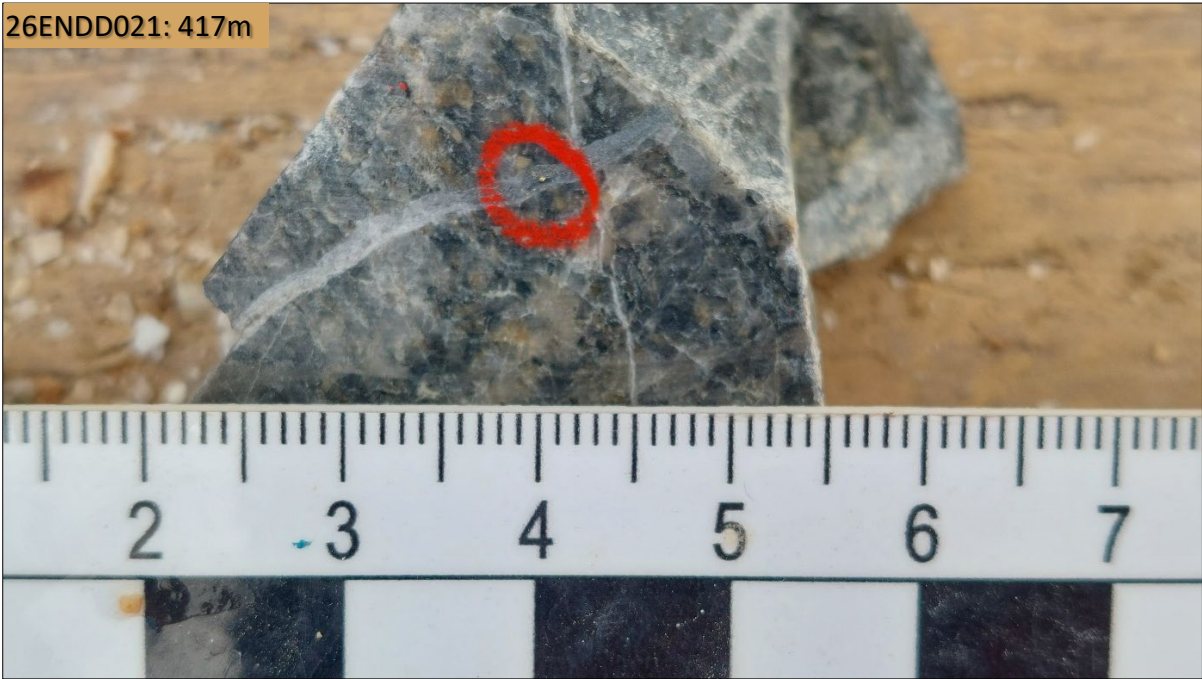
Photo 2. Visible gold (circled red) in hole 26ENDD021 at 417m down hole in a fine quartz-carbonate-sulphide veinlet with weakly phyllic altered crackled brecciated granite. Numerical units on scalebar are centimetres.
