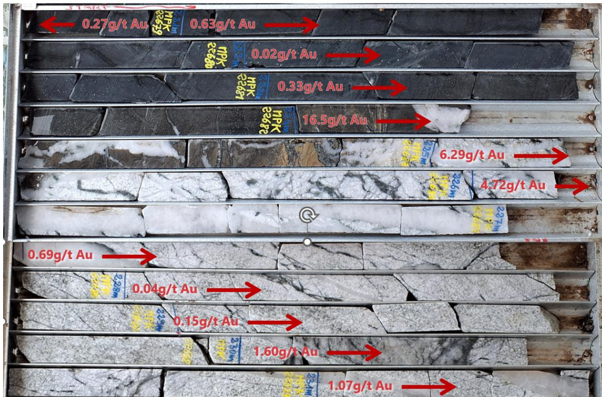
Figure 7 | FNDC038, 220.8m to 231.5m photo Interval to illustrate mineralisation style – Assay Interval 221m to 232m averages 11m @ 2.91g/t gold, located at the upper contact to the mineralised intrusion body, within the reported significant intercept of .74.5m @ 1.67g/t gold from 221m depth, including 29m @ 3.46g/t gold from 224m depth (ASX announcement 15 July 2025 & Refer to Figure 4 for cross section)
