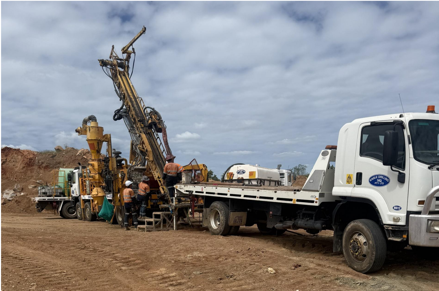
Figure 7: Diamond drilling North Central pit.
