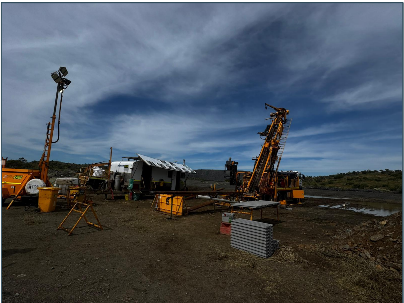
Figure 1: Multi-purpose (Diamond / RC) drill rig onsite at Barbara Copper-Gold Project, 18 th April 2026
