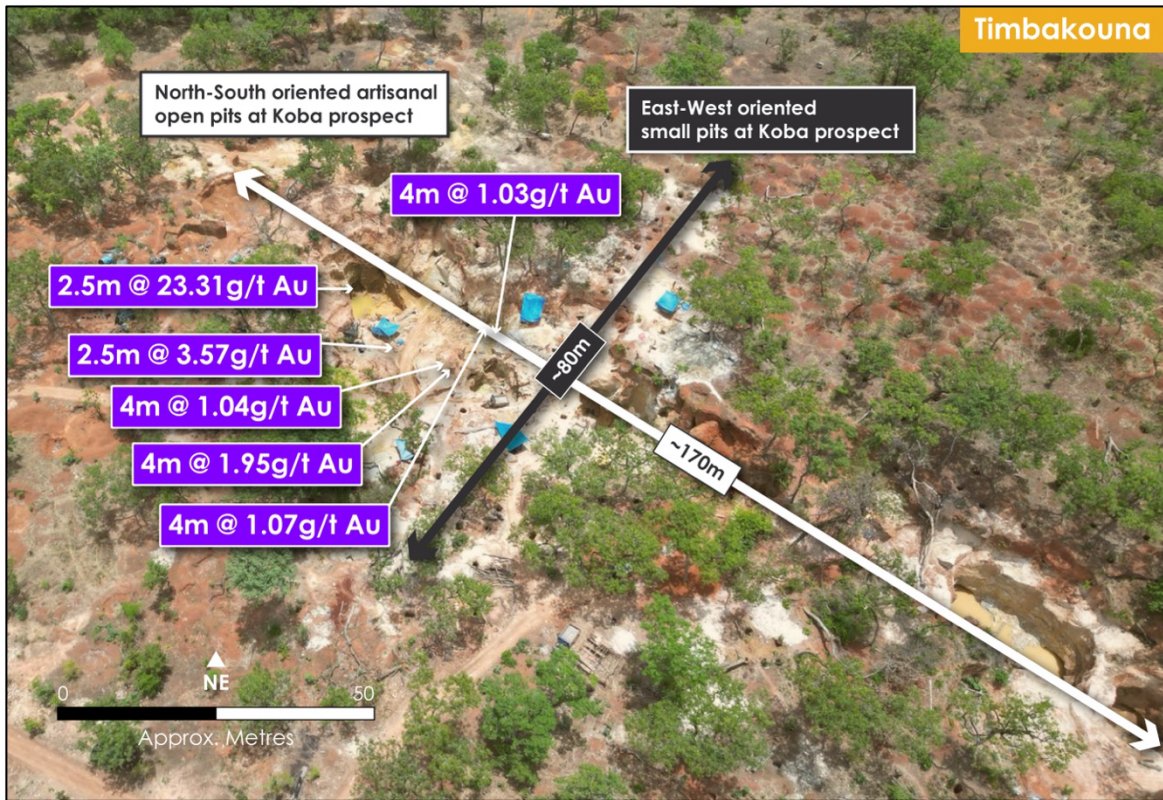
Figure 2: Artisanal workings at the Koba Prospect, Timbakoua, highlighted by north-south and crosscutting east-west structures with channel sampling from within artisanal workings producing gold grades of up to 2 m at 23.21g/t Au.
