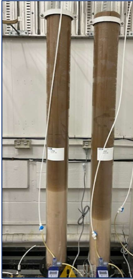
Figure 2. CLT-01 and CLT-02 in progress at Core Resources' laboratory. 16-day operating photo showing both full columns in operation.
