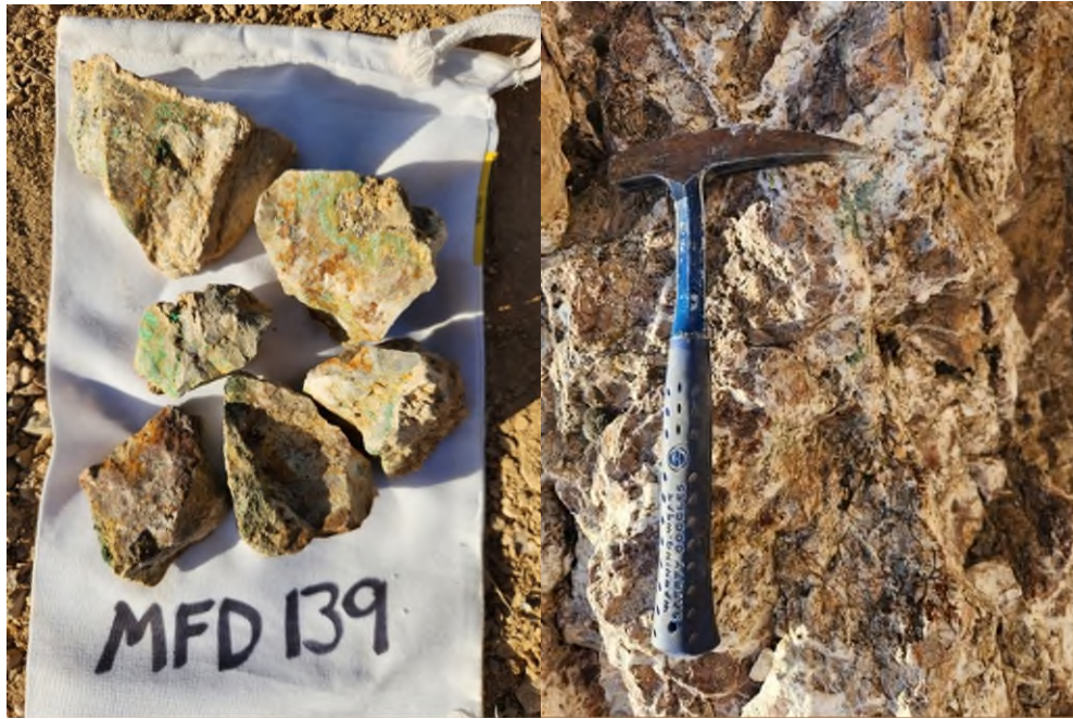
Figure 1 - Sample Site of MFD139 (534 g/t Ag, 0.19% Sb, 0.5% Cu. Image on right taken from sample site, showing ferruginised vein breccia
