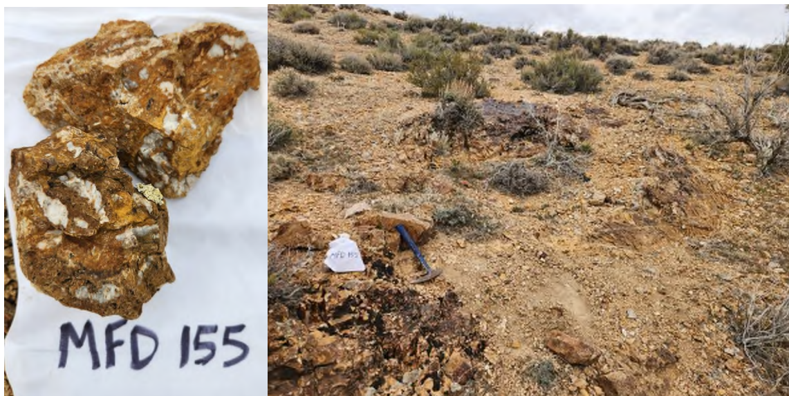
Figure 3 - Samples KFD155 (1.04 g/t Au) and sample site showing brecciated and ferruginous outcrop
