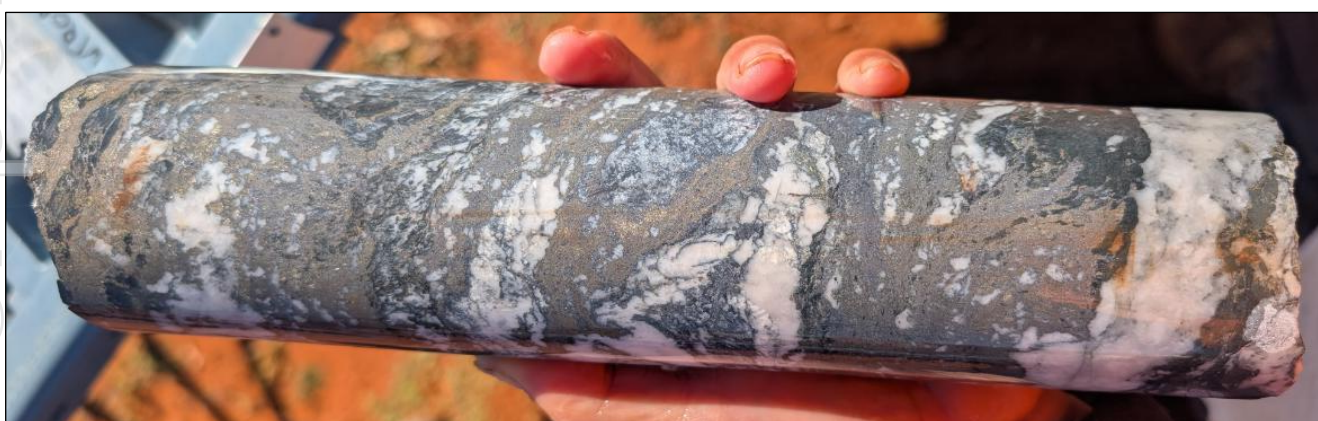
Figure 1 – Semi-massive/stringer sphalerite-galena-pyrite mineralisation @ 546.3m down-hole
