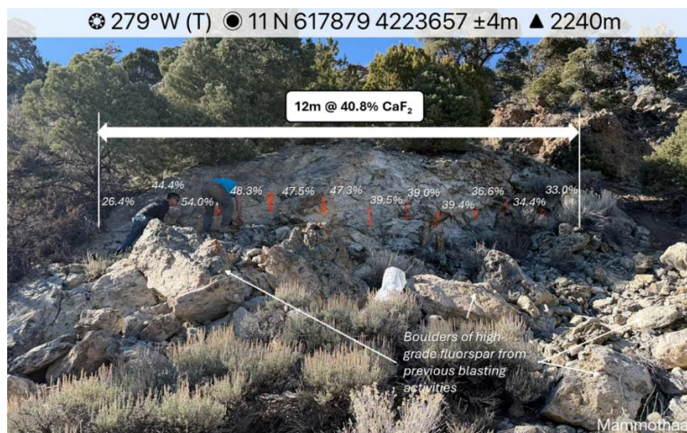
Figure 4: View west of the outcrop of the channel sampling at Mammoth. Orange paint marks indicate 1m samples. The full extent of the outcrop was sampled.
