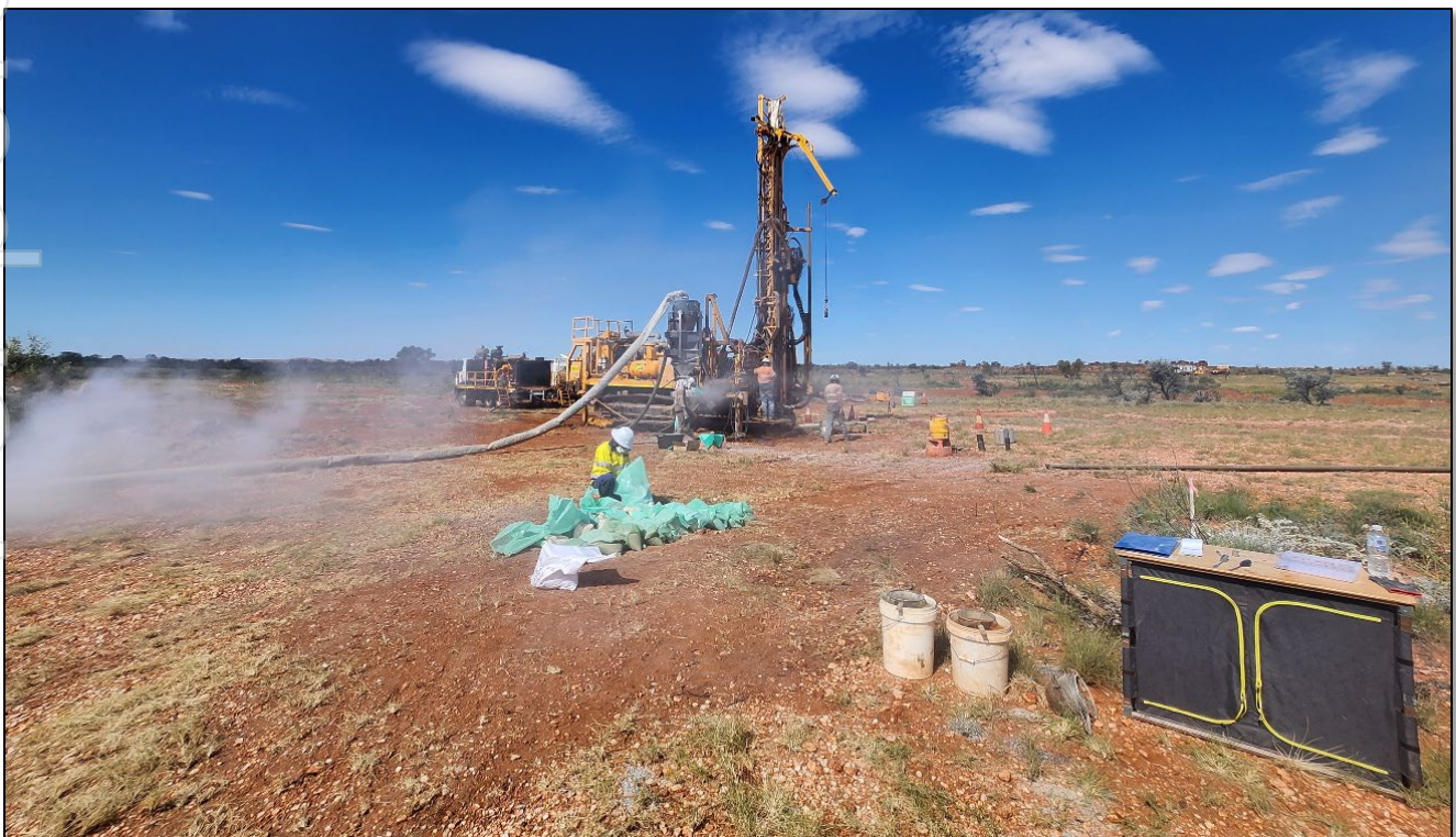
Figure 5: RC drilling at Tiger 2 Prospect, Marble Bar gold Project
