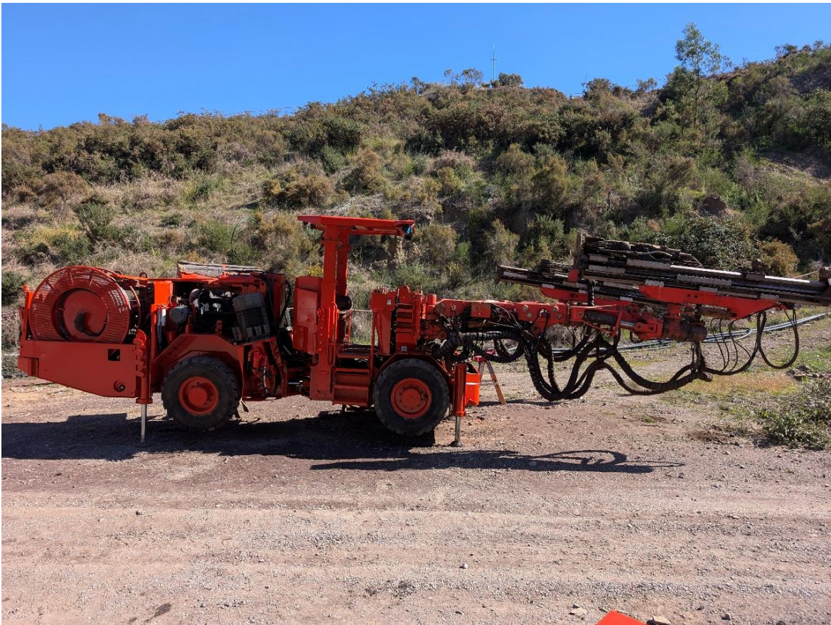
Figure 3. Jumbo ready for work
