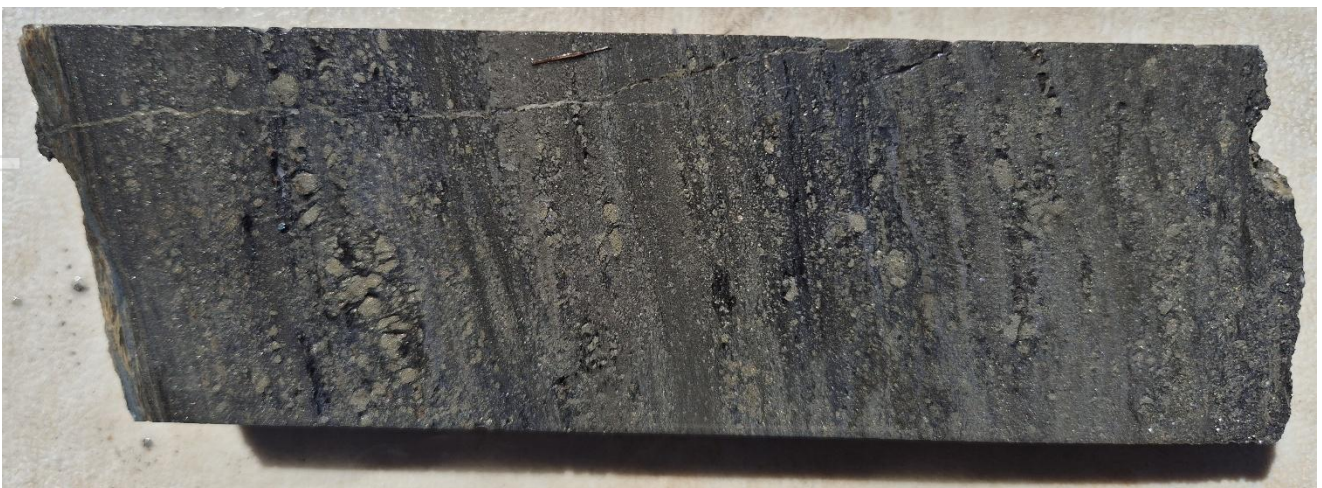
Figure 1: HQ3 drill core from hole CMKNI001 (Sample ID 162512), showing massive sulphide mineralisation from 98m, which returned 0.5m @ 9.7 g/t Au, 90 g/t Ag, 11.5% Zn, 5.0% Pb and 0.3% Cu .
