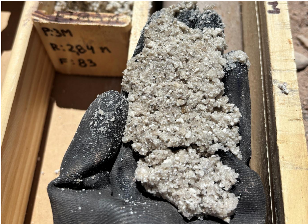
Figure 4. Core from (284m-287m): Unconsolidated, medium to coarse sand matrix, matrix-supported, with sub-angular clasts. Very high porosity from well six.
